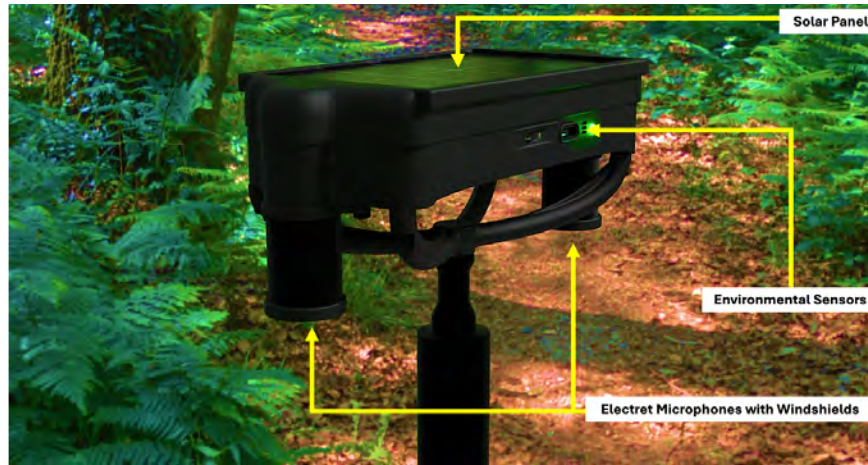
Figure 4.12: BuzzCam with sensor locations shown. The system can be mounted to a standard tripod so the height is adjustable [56].
