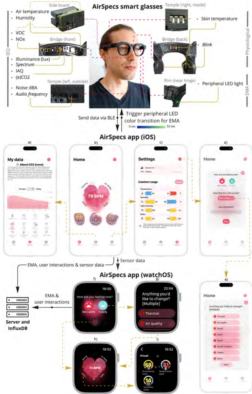
Figure 3.3: System overview of AirSpecs device and apps [30]. The sensor readings of the device in the top figure (except those in italic ) are accessible by the user. Most readings are presented in raw form, except that skin temperature data was used to estimate cognitive load. Screenshots of the AirSpecs apps design in iOS and the corresponding watchOS are shown, including home, historical records, settings, and the survey. The watchOS app aims to provide spontaneous information, so we eliminated the historical records and settings screens in its design. Two sets of sensors that measure air temperature, humidity, VOC, and NO x are located in the left temple (on a sideboard) and bridge, considering that measurements near the breathing area and the surrounding environment can differ [5]
