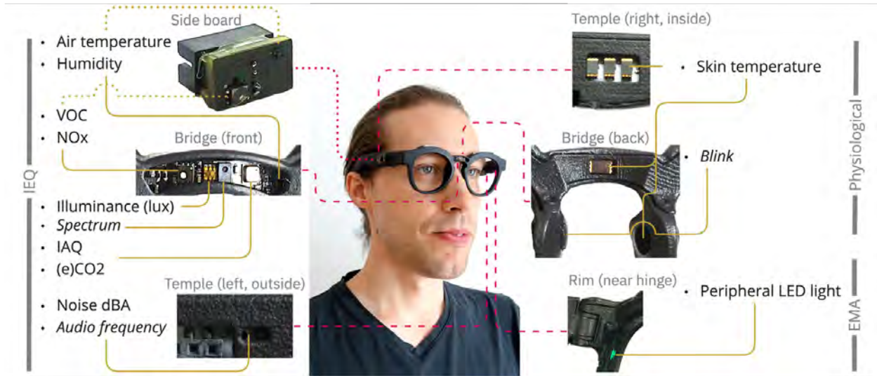
Figure 3.2: Labeled overview of sensors in the AirSpecs Smarteyeglass Platform [30]
